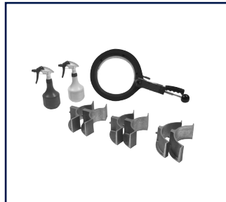
MPC-xxx Manual Pipe Cutter
